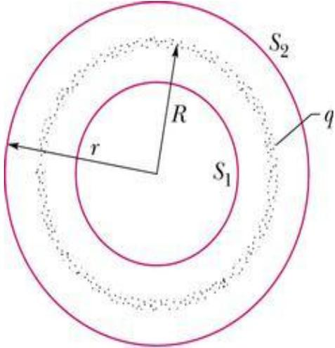
The diagram shows a spherical shell of radius  $R$  with a total charge  $q$  distributed uniformly on its surface. Two concentric Gaussian surfaces are shown: an inner surface  $S_1$  with radius  $r$  (where  $r < R$ ) and an outer surface  $S_2$  with radius  $R$ . The shell is represented by a ring of small dots.
